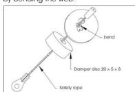
Then run the preassembled rope through an elongated hole (in the area of the later fastening points of the safety rope) in the rail channel out of the ceiling void downwards.  When assembling the LOOP® elements, the safety rope is screwed to the LOOP® element by means of a wing nut.
