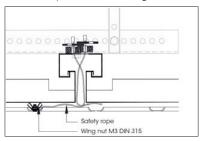
. Measure the position of the LOOP® element exactly using the laser (longitudinal and transverse rows). Hold the LOOP® element with the rear magnet (20 pieces per standard element) from below horizontally against the ceiling S7 KS (friction force by magnet). For the arrangement of the magnets, see below. To simplify assembly/disassembly, the magnets can be glued to the LOOP® element (e.g. LOCTITE).
